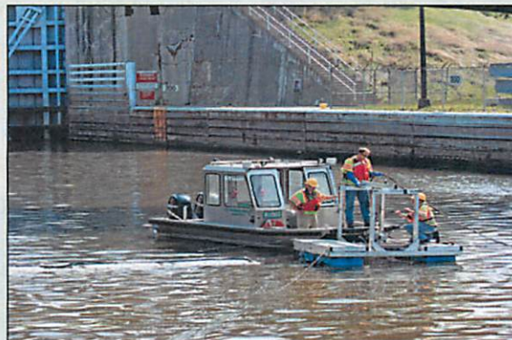
USGS scientists measuring flow velocity in a lock channel.
